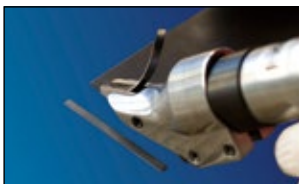
▲ Operation of Air Metal Shear
