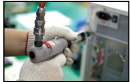
▲ Operation of Auto Shut-Off Screwdriver
