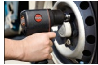
▲ Operation of 1/2" Impact Wrench with Torque Controlled
