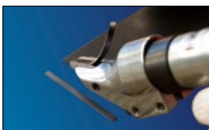
▲ Operation of Air Metal Shear
