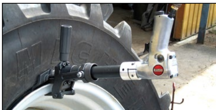
▲ Operation of Bead Breaker
