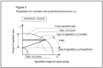
The proper selection of regulated pumps is shown in figures 3, 4 and 5. (Comparison of pump's characteristics determined by the design with actual technical characteristics of a particular pump).
