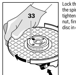
Lock the grinder spindle with the spindle lock button 1. To tighten the quick-clamping nut, firmly turn the grinding disc in clockwise direction.
