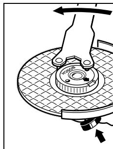
A properly attached, undamaged quick-clamping nut can be loosened by hand when turning the knurled ring in an anticlockwise direction.
