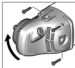
The machine head can be rotated with respect to the machine housing in 90° steps. In this manner, the On/Off switch can be brought into a more convenient position for special working situations, e.g., for cutting operations using the cutting guide with dust extraction protection guard **18** or for left-handed persons.
