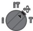
Vario-Lock position for adjustment of the chiselling position The mode selector switch 9 does not latch in this position.
